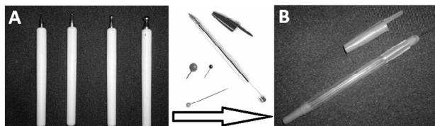
**Figure 1.** The iron pens (1, 2, 4 and 7 mm) used to design the figures of the fungus in high thickness. By using pins and common pens we may produce these iron pens or stylets (B) that increase the touch sensitiveness of the drawings.
