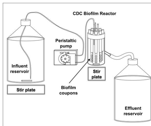
**Figure 2. Experimental set-up of a flow-through drinking water reactor system used in the persistence experiments.**
