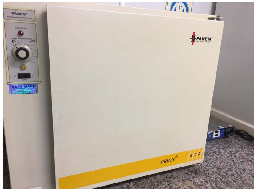
**Figure 3.** Fanem Orion 520 greenhouse, temperatures from 50°C to 250°C, 62 L volumetric capacity.
