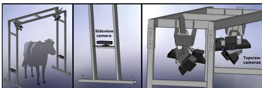
Figure 1. True to scale technical drawing of the recording unit. Left: A framework was equipped with six Kinect cameras. Middle: On each side one Kinect camera was mounted in sideview position. Right: Pairs of Kinect cameras were fixated in topview positions.
