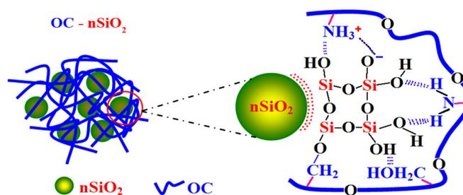
**Figure 2.** Schematic illustration of interactions between OC and  $n\text{SiO}_2$ .
