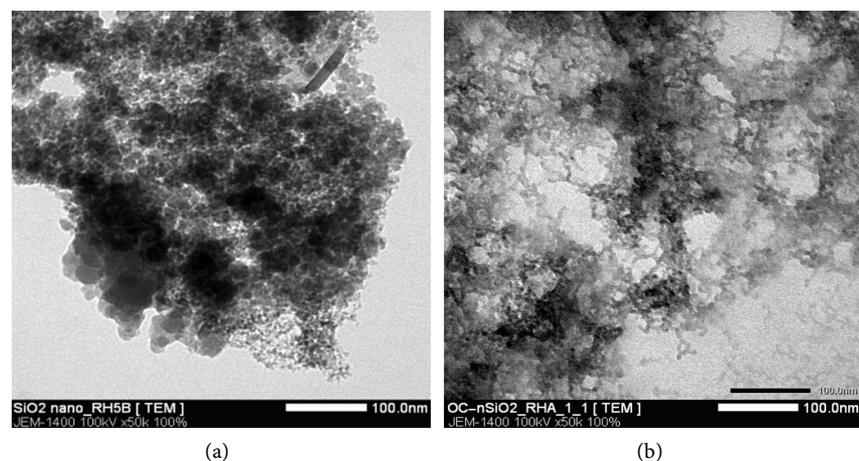
**Figure 1.** TEM images of nSiO<sub>2</sub> (a) and nSiO<sub>2</sub> in mixture of 1% OC - 1% nSiO<sub>2</sub> (b).
