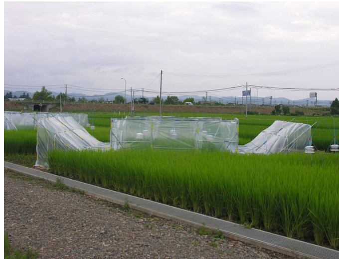
Figure 3. Example of the OTC-SDF2 field settings. Scenario 3 is shown, in which the apparatus was set approximately 30 degrees from the perpendicular direction. Thus, the right funnel is facing 10 degrees east of north. The temperature sensors inside and outside the OTC-SDF2 were covered with 5 radiation shield layers.
