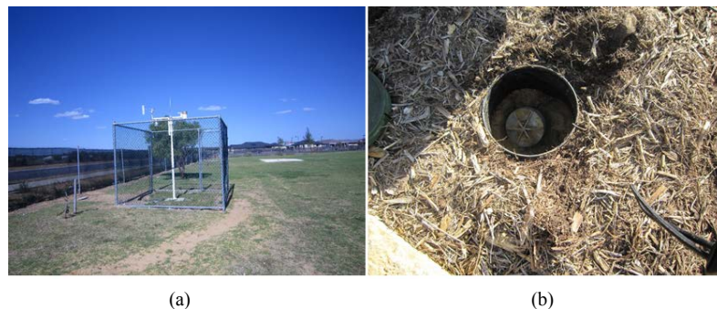
Figure 2. A local meteorological station (a) and soil moisture sensor (b) associated with the third-pipe irrigation system in “The Green”.
