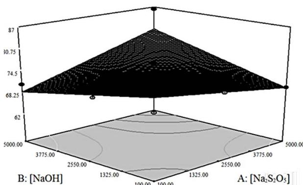
Figure 3. 3D surface of carbohydrate content using the screw press.
