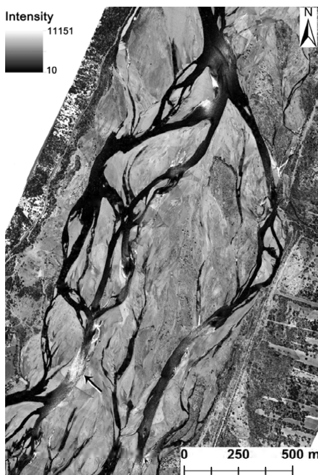
Figure 3. LiDAR intensity raster of Cornino sub-reach in 2011. The arrow indicates an area with anomalous intensity values.
