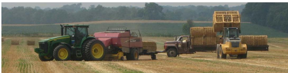
**Figure 1.** The large square baler, bale handler, and bale truck used in straw harvesting.
