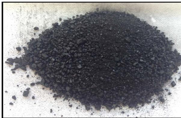
**Figure 1.** Image of the fabricated Co-Fe<sub>2</sub>O<sub>3</sub> powder.
