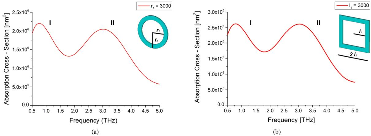
**Figure 2.** Absorption cross-section spectrum for (a) circular ring with  $r_1 = 3000$  and  $r_2 = 4000$ , and (b) square ring with  $l_1 = 3000$  and  $l_2 = 4000$ .
