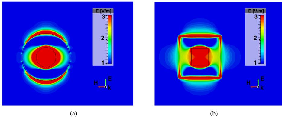
**Figure 3.** Near electric field distribution of (a) circular ring at 1.5 THz with  $r_1 = 1661$  and  $r_2 = 4000$ , and (b) square ring at 1.4 THz with  $l_1 = 1661$  and  $l_2 = 4000$ .
