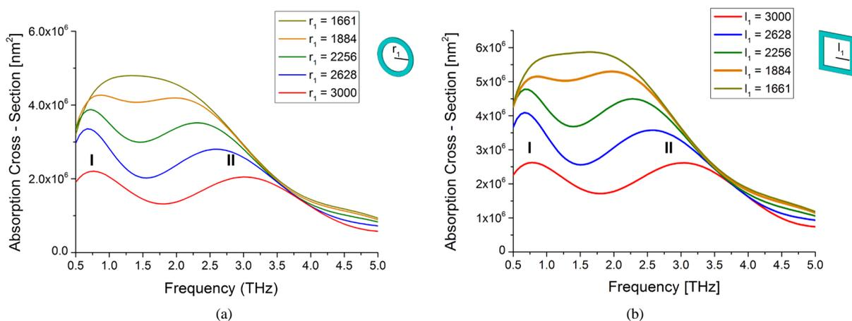
**Figure 4.** Absorption cross-section spectra for (a) circular ring by vaying  $r_1$  with  $r_2 = 4000$ , and (b) square ring by varying  $l_1$  with  $l_2 = 4000$ .
