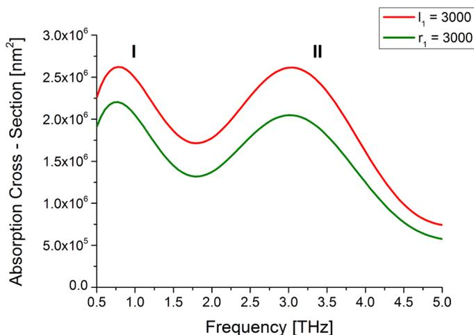
**Figure 5.** Absorption cross-section spectra for circular ring (green color) with  $r_1 = 3000$  and  $r_2 = 4000$  and square ring (red color) with  $l_1 = 3000$  and  $l_2 = 4000$ .
