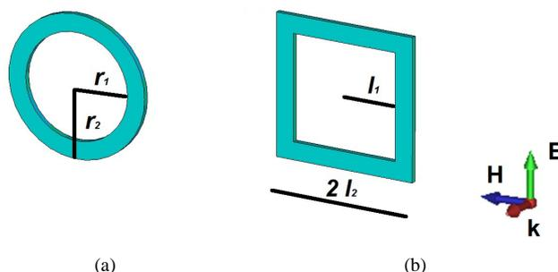
**Figure 1.** Geometrical sketch of the particles under study: (a) Circular ring; (b) Square ring.
