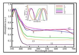
Figure 9. Optical absorption spectra of various QDs ZnO nanorods (samples 5, 13, 2, 12) and nanosphericals (samples 3, 11).
