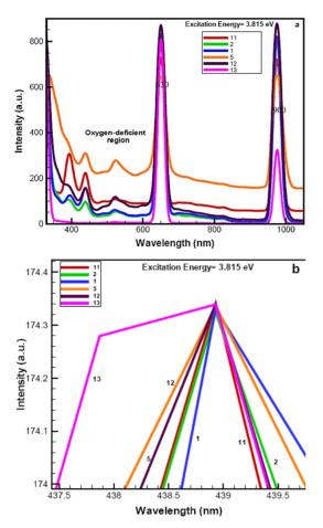
Figure 11. Photoluminescence spectra of (a) various QDs ZnO NPs and (b) the inset shows expansion of limited 437 - 439 nm wavelengths for illustration of broad, ladder and wave-like peaks of especial point defects. All of the products have 620 and 900 nm wavelength in (a) curve.
