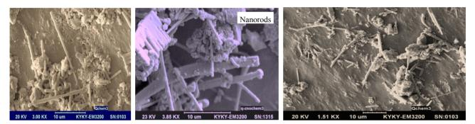
Figure 1. SEM images of QDs ZnO nanorods for sample 1.
