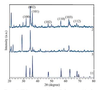
Figure 7. XRD patterns of three ZnO nanoparticles for nanorods of samples 2 and 5 and nanospherical of sample 11.
