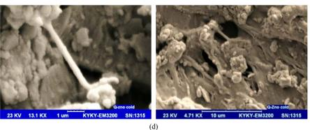
Figure 6. SEM images of various ZnO nanostructures for (a) ZnO QDs of sample 8; (b) sample 10; (c) sample 11 and (d) ZnO QDs as nanorods (nanotubes) for sample 12.
