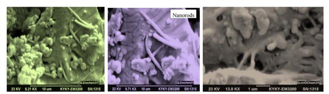
Figure 2. SEM images of QDs ZnO nanorods for sample 2.
