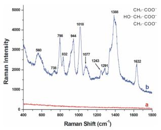
Figure 3. SERS spectra of citrate group in the concentrated  $10 \times Ag$ -NPs solutions (a) and (b) with one cycle of ultrapure water dilution, centrifugation, removing the supernatant and then ultrasonication for  $10 \times Ag$ -NPs.
