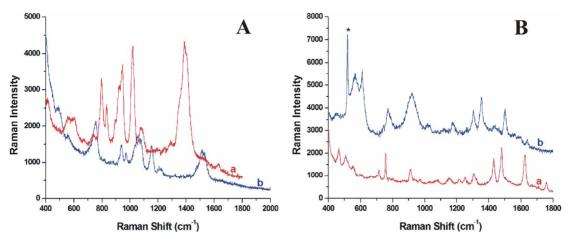
Figure 6. Comparison of SERS spectrum of citrate anions (A) and R6G (B) in the Ag-NPs aggregation aqueous solution (a) or the dried Ag-NPs aggregation on the Si substrate (b). The symbol of \* in this figure denotes the Raman signal from Si substrate.
