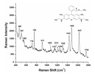
Figure 5. SERS spectrum of R6G in the Ag-NPs aggregate solution with one cycle of ultrapure water dilution, centrifugation, removing the supernatant and then ultrasonication for  $10 \times \text{Ag-NPs}$ .
