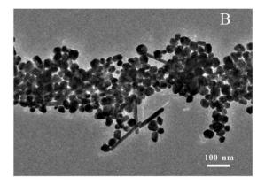
Figure 2. (A) UV-Vis-NIR spectra of an original citrate-reduced Ag-NPs solution (a, Ag-blank), and Ag-NPs aggregated solutions after one cycle (b, Ag-1), two cycles (c, Ag-2), three cycles (d, Ag-3), and four cycles (e, Ag-4) of centrifugation, removing the supernatant, ultrasonication and water dilution, respectively; (B) TEM image of the Ag-NPs aggregation after two cycles of the treatment process of centrifugation, ultrasonication and water dilution.
