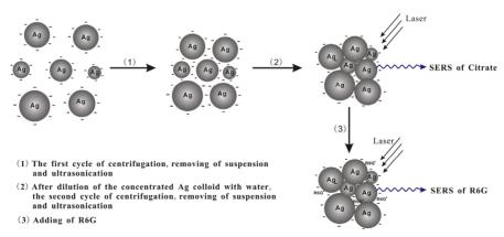
Scheme 1. Schematic illustration of the aggregating process of Ag-NPs by the proposed method and used as the substrate for SERS analysis of citrate and R6G.
