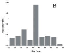
Figure 1. (A) TEM image of the original citrate-reduced Ag-NPs prepared by the present method; (B) The size distribution of Ag-NPs with polydispersity.
