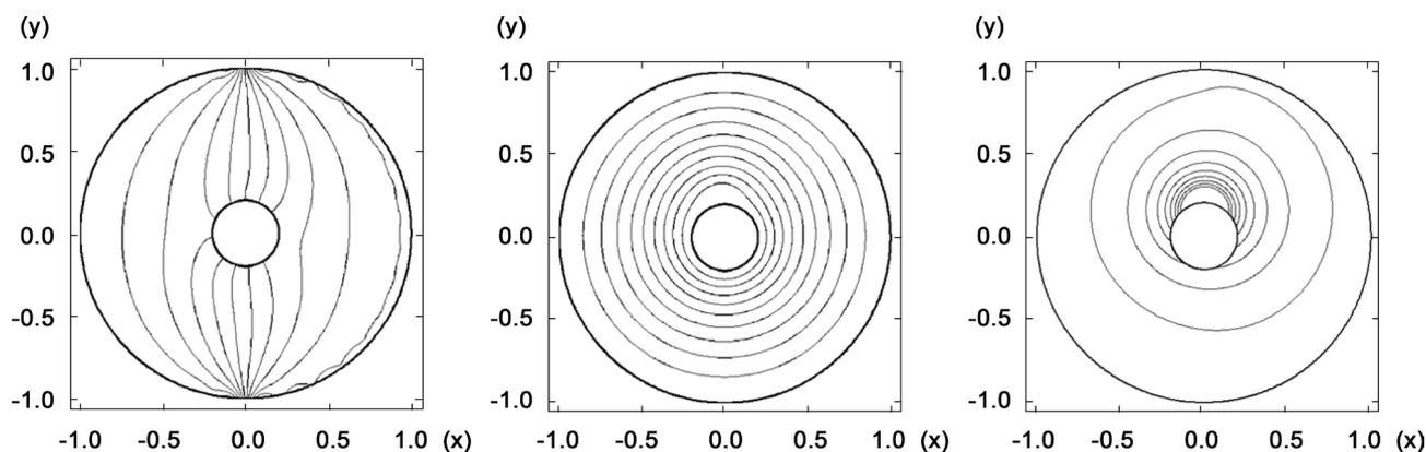
**Figure 4.** Isotherms (at an interval of 0.1), streamlines (at an interval of  $1.0 \times 10^{-7}$  stream function) and dimensionless magnetization field strengths (at an interval of  $2.0 \times 10^{-3}$  with from 0.002 to 0.02) in the case of the electric current wire fixed at  $(x, y) = (0, 0.15)$ , where the direction of flow is clockwise.
