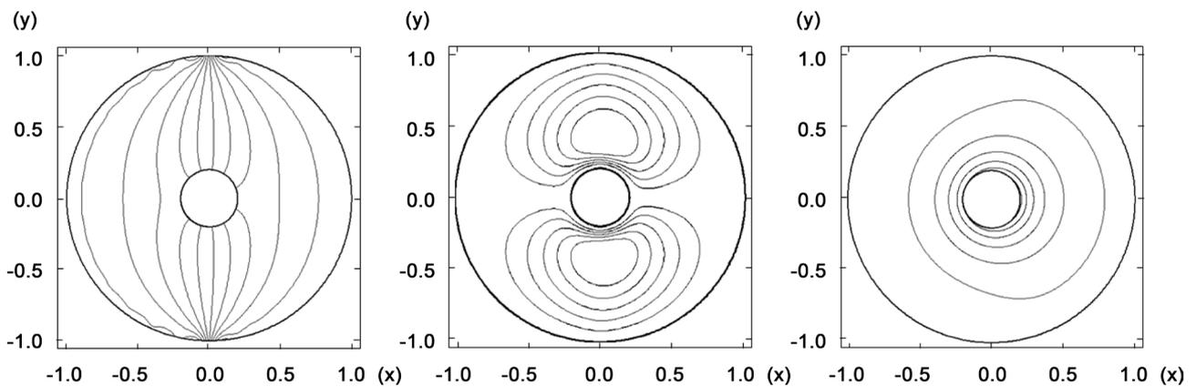
**Figure 2.** Isotherms (at an interval of 0.1), streamlines(at an interval of  $1.0 \times 10^{-7}$  stream function) and dimensionless magnetization field strengths (at an interval of  $1.0 \times 10^{-3}$  with from 0.001 to 0.007) in the case of the electric current wire fixed at  $(x, y) = (0, 0)$ , where the direction of velocity along the center is leftward.
