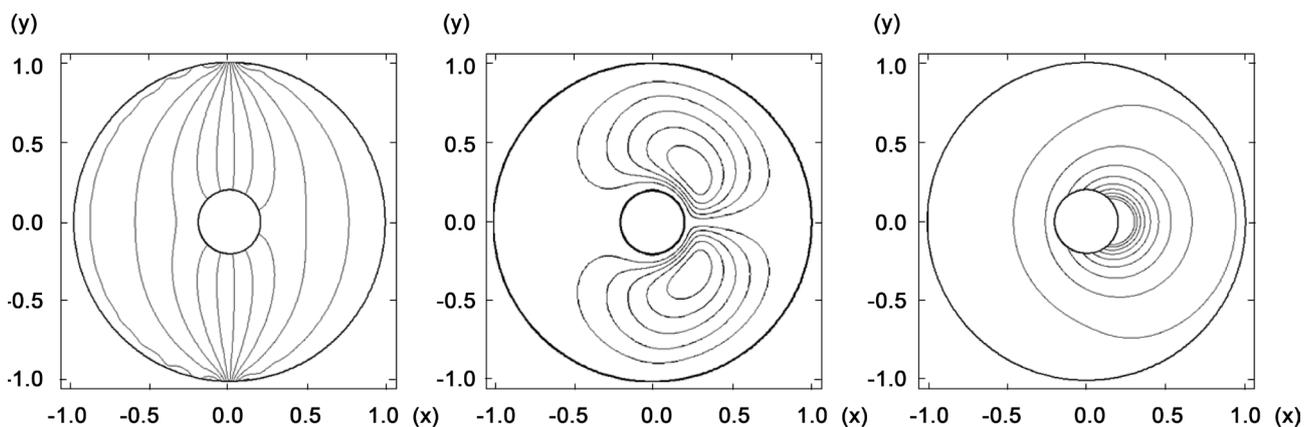
**Figure 3.** Isotherms (at an interval of 0.1), streamlines (at an interval of  $2.0 \times 10^{-8}$  stream function) and dimensionless magnetization field strengths (at an interval of  $2.0 \times 10^{-3}$  with from 0.002 to 0.02) in the case of the electric current wire fixed at  $(x, y) = (0.15, 0)$ , where the direction of velocity along the center is leftward.
