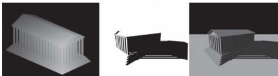
Figure 2. The far left image is a shadow map—the contents of the z -buffer as rendered from the point of view of a particular light source. The pixels of the center image are black where the light-space depth test failed (fragment in shadow) and white where it succeeded (fragment not in shadow). The far right image shows the final scene rendered with shadows.
