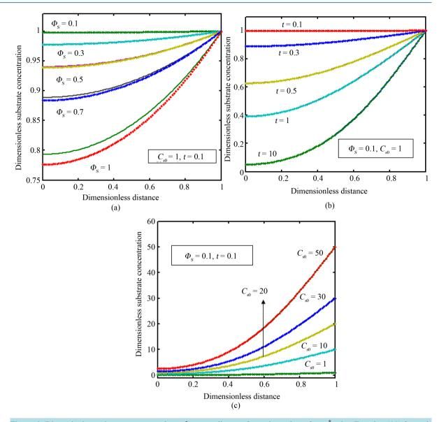
**Figure 2.** Dimensionless substrate concentration  $c_s^*$  versus distance from electrode surface  $z^*$  using Equation (11) for various values of parameters  $\Phi_s$ , *t* and  $c_{s0}$ .
