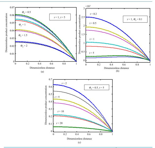
**Figure 3.** Dimensionless product concentration  $c_p^*$  versus distance from electrode surface  $z^*$  using Equation (12) for various values of parameters  $\Phi_s$ , *t* and *r*.
