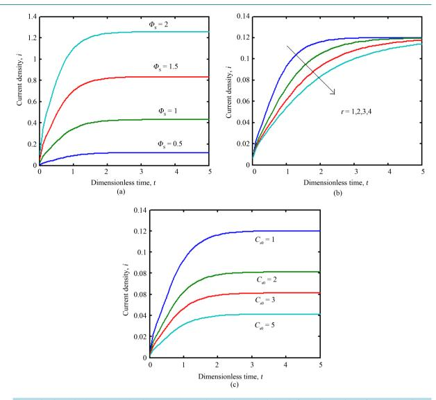
**Figure 4.** Dimensionless current density  $i/nFD_p$  versus time *t* using Equation (14) for various values of parameters  $\Phi_s$ ,  $c_{s0}$  and *r*.
