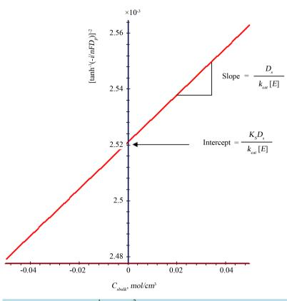
**Figure 5.** A plot of tan  $h^{-1}(i/nFD_p)^{-2}$  versus initial substrate concentration  $C_{Sbulk}$  using Equation (17) to estimate the kinetic parameters.
