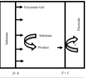
Figure 1. Schematic model of an enzyme-membrane electrodes.
