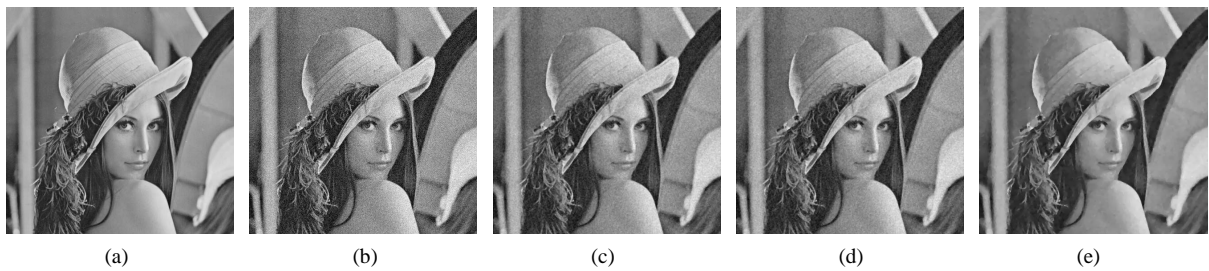
Figure 4. The contract of de-noising for three methods to image Lena. (a) Original image; (b) Noisy image; (c) De-noising image by mean filter; (d) De-noising image by median filter; (e) De-noising image by Sobel-TV.
