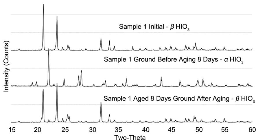
**Figure 2.** Three XRD scans for Sample 1 initially after drying (top scan), and Sample 1 after grinding then drying for 8 days (middle scan), Sample 1 that was dried for 8 days before grinding (bottom scan).
