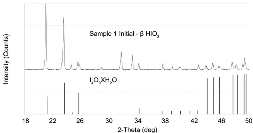
**Figure 3.** Diffraction pattern from XRD for Sample 1 (Black). Blue curves from PDF #00-045-0872 indicating 2-Theta and relative intensity of  $I_4O_9XH_2O$ .
