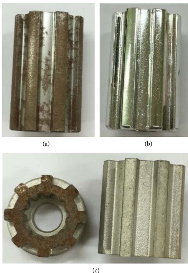
**Figure 1.** Comparison of sintered stainless steel parts and pack-chromizing treated sintered steel parts. (a) Sintered stainless steel, (b) Al sputtering sintered stainless steel, (c) pack-chromizing treated sintered steel.
