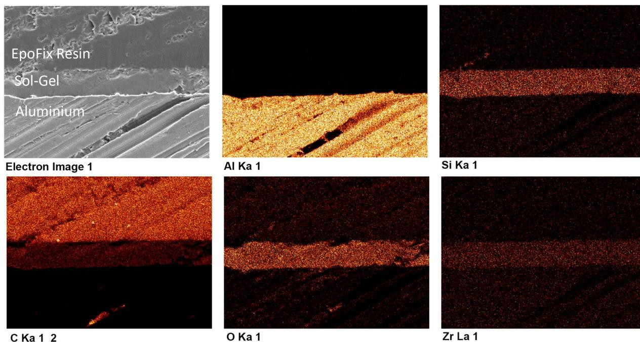
**Figure 6.** SEM micrograph and element map of sol-gel material A coated onto AA2024-T3, encased in EpoFix resin.
