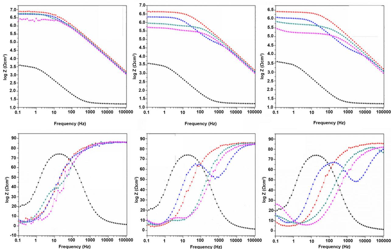
**Figure 7.** Bode plots of coatings A (red), B (blue), C (green) and D (purple) after 1, 24 and 48 h (left to right) of exposure to Harrison's solution.
