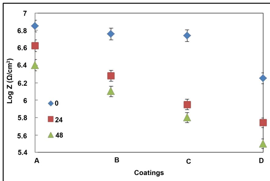
**Figure 8.** Impedance values for coatings A to D at a frequency of 0.1 Hz, for exposure times of 1, 24 and 48 h to Harrison's solution.
