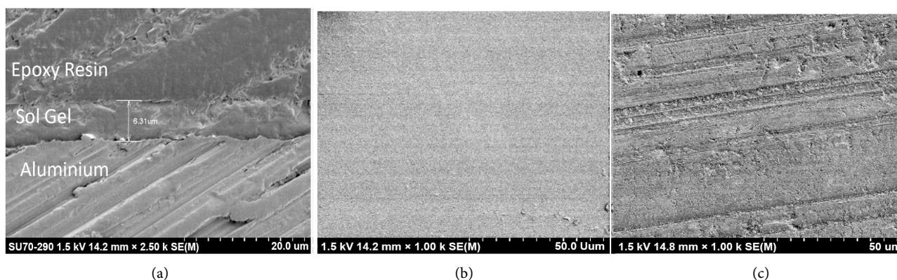
**Figure 5.** SEM images of cross-section (a) and top view (b) of sol-gel A deposited on an AA2024-T3 aluminium substrate, and (c) an SEM image of the bare AA2024-T3 surface.
