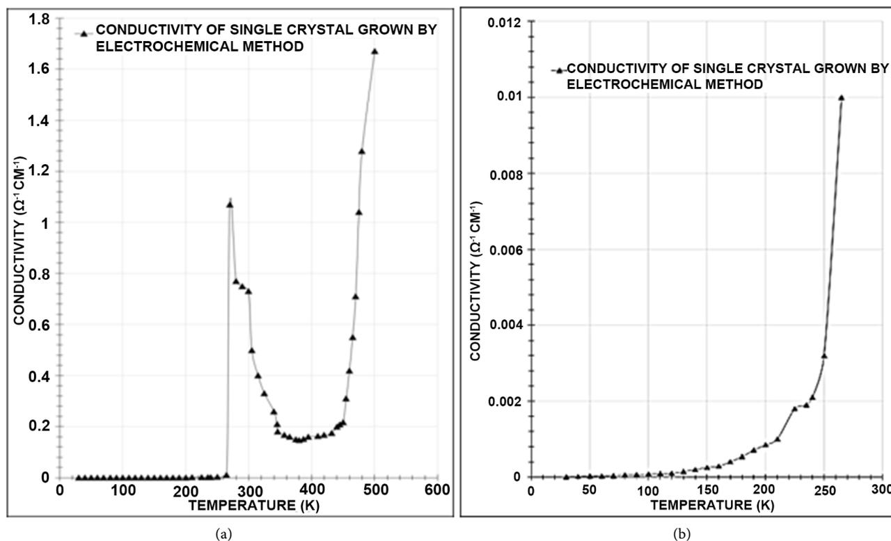
**Figure 1.** (a) Plot of conductivity as a function of temperature in the region 30 to 500 K for K-TCNQ single crystal grown by electrochemical method; (b) Plot of conductivity as a function of temperature in the region 30 to 265 K for K-TCNQ single crystal grown by electrochemical method.
