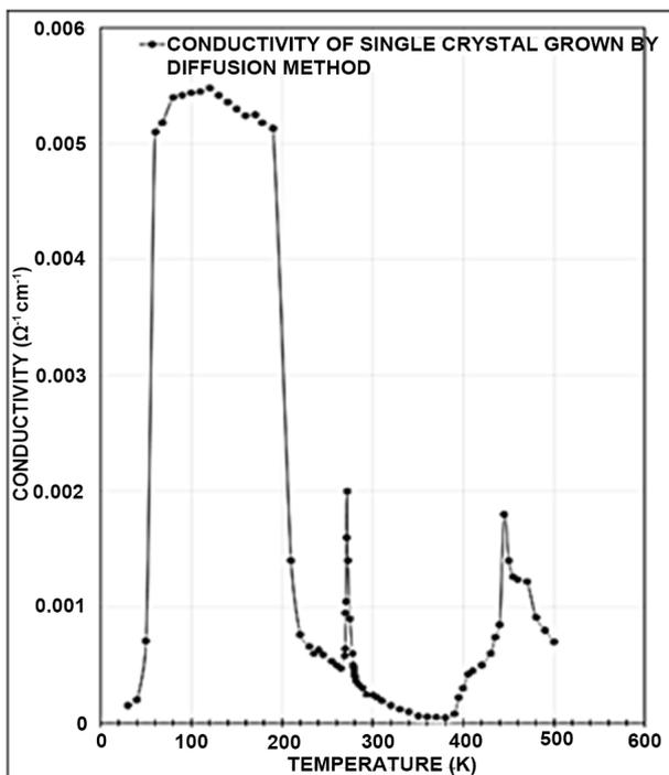
**Figure 3.** Plot of conductivity as a function of temperature in the region 30 to 500 K for K-TCNQ single crystal grown by diffusion method.
