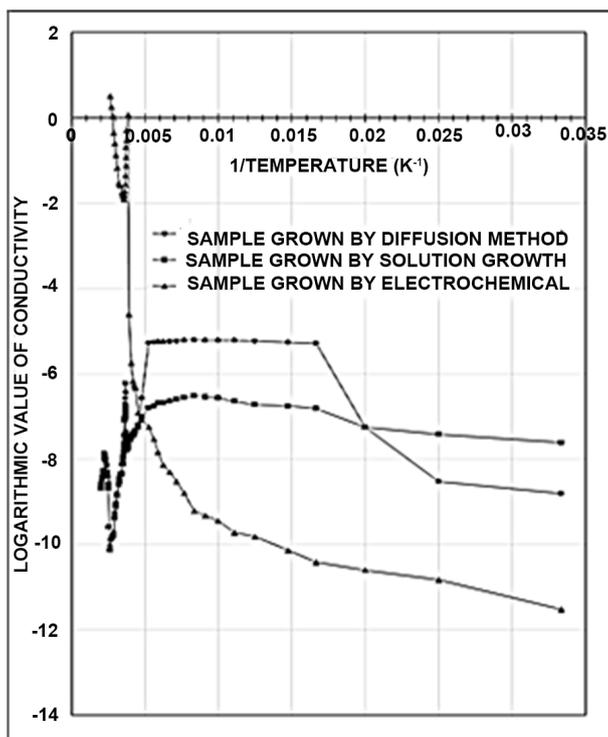
**Figure 5.** Plot of logarithmic value of conductivity against  $1/\text{temperature}$  in the region 30 to 500 K for K-TCNQ single crystal grown by diffusion method.
