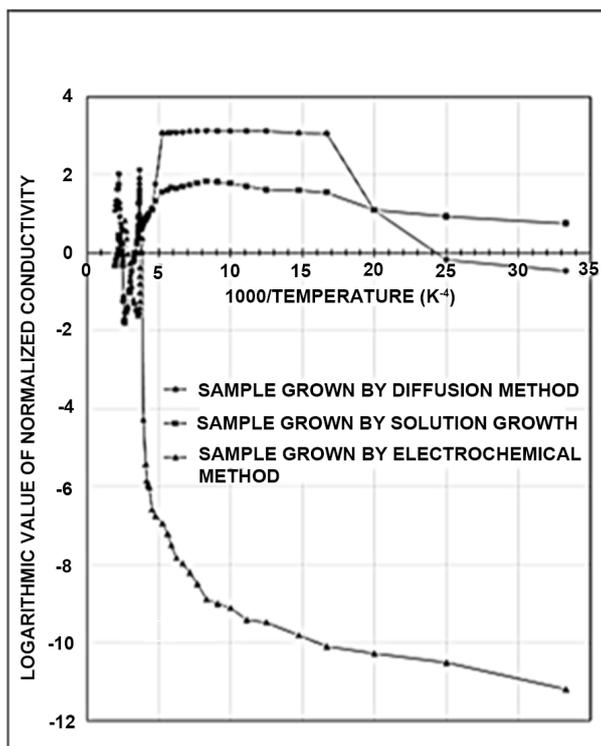
**Figure 4.** Plot of logarithmic value of normalized conductivity as a function of  $1000/\text{temperature}$  in the region 30 to 500 K for K-TCNQ single crystal grown by diffusion method.
