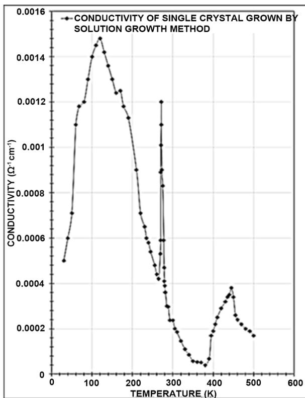
**Figure 2.** Plot of conductivity as a function of temperature in the region 30 to 500 K for K-TCNQ single crystal grown by solution growth method.
