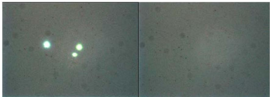
Figure 6. The plasma flash in the film and its surface morphology after flash during laser conditioning process.
