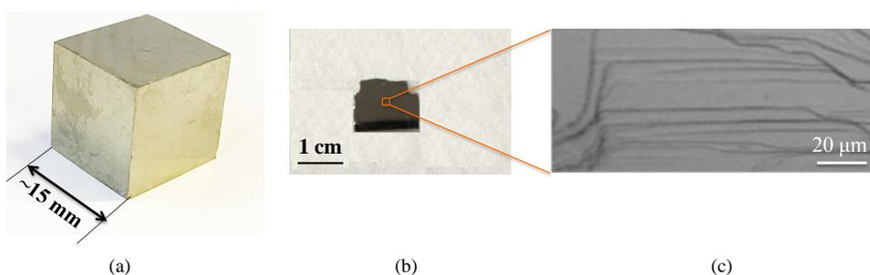
**Figure 2.** (a) Image of natural pyrite mineral (Navajun, Spain); (b) Image of pyrite substrate after cutting; (c) Optical microscope image of the outermost surface of the pyrite showing the step-like structure of single crystal planes.
