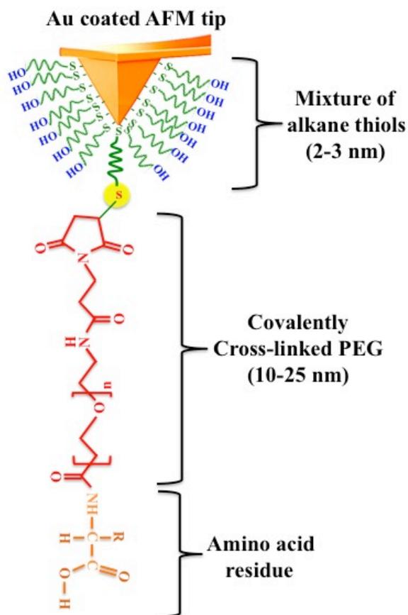
**Figure 1.** Schematic AFM tip modification by amino acid residues. Gold-coated AFM tip with nominal radius of  $\sim 20$  nm was chemically modified by amino acid molecules through MAL-PEG<sub>n</sub>-NHS cross-linker. The maleimide group reacts with sulfhydryls to form stable thioether bonds. The N-hydroxysuccinimide ester (NHS) group reacts specifically with N-terminal amino groups at pH = 7 - 9 to form stable amide bonds.
