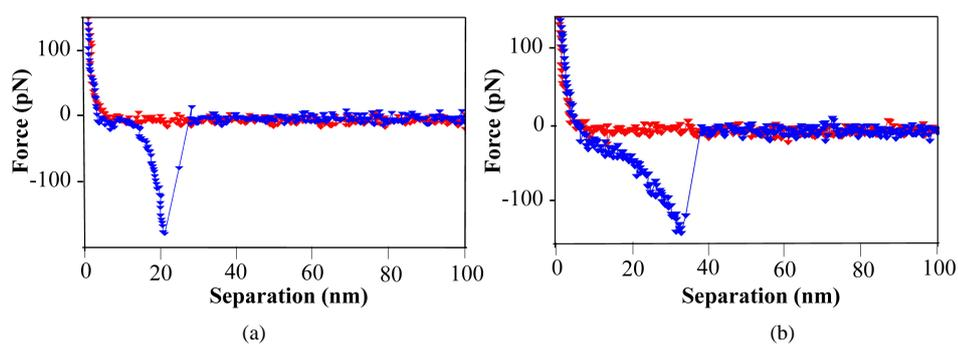
**Figure 8.** Specific adhesion force curve of an AFM tip modified with (a) methionine and (b) cysteine on pyrite surfaces. The red and blue traces indicate the signal upon approach and retraction from the surface, respectively.
