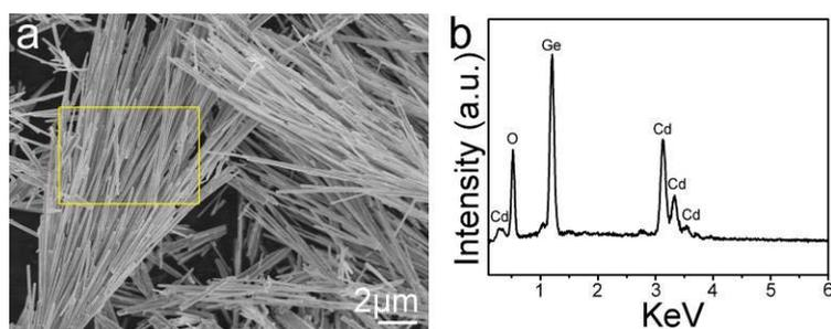
**Figure 5.** (a) A SEM image of the  $\text{Cd}_2\text{Ge}_2\text{O}_6$  nanowires. The section in the yellow rectangle was taken for data collection; (b) Energy dispersion X-ray spectrum of the as-prepared product.
