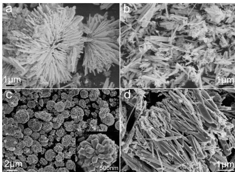
**Figure 2.** SEM images of the  $\text{Cd}_2\text{Ge}_2\text{O}_6$  products synthesized at  $180^\circ\text{C}$  for 24 h with (a) EDA; (b) PVP; (c) SDBS and (d) CTAB added as surfactant.
