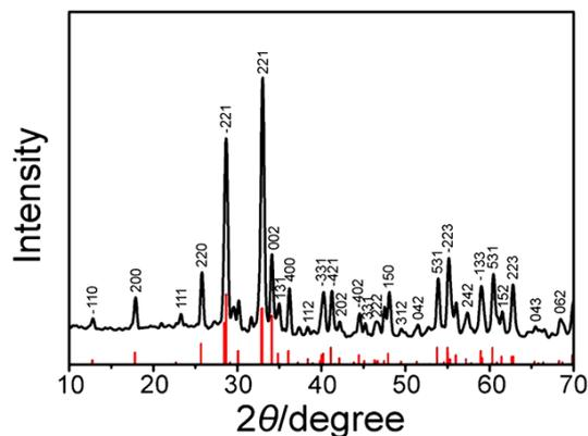
**Figure 4.** XRD pattern of the as-synthesized  $\text{Cd}_2\text{Ge}_2\text{O}_6$  product prepared using  $\text{GeO}_2$  and  $\text{CdO}$  as the precursors.
