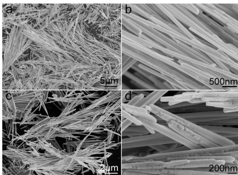
**Figure 3.** SEM images of the as-synthesized products with the molar ratio of  $\text{GeO}_2$  to  $\text{CdO}$  of (a) 2:1 and (b) 1:1. CTAB was added as surfactant.
