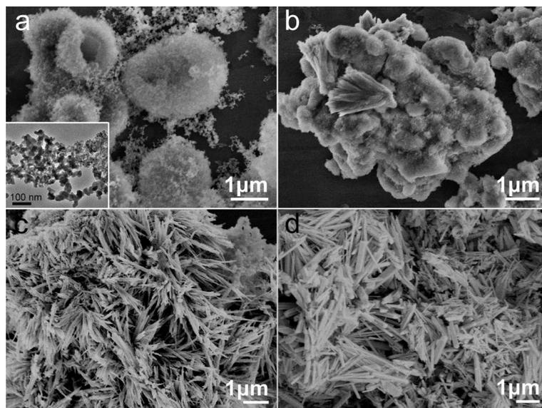
**Figure 1.** SEM images of the as-synthesized products that were carried out at (a) 120°C; (b) 140°C; (c) 160°C and (d) 180°C for 24 h. The inset is the high magnified TEM image of the nanoparticles.
