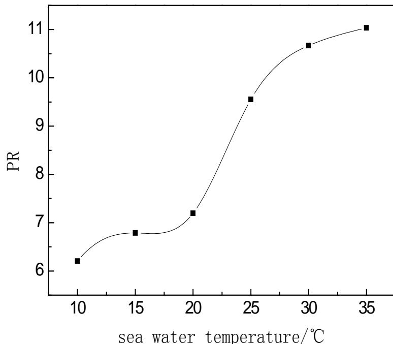
Figure 3. Effect of feed seawater temperature on the PR.
