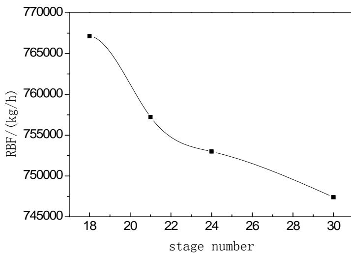
**Figure 8. Effect of flash stage number on RBF.**
