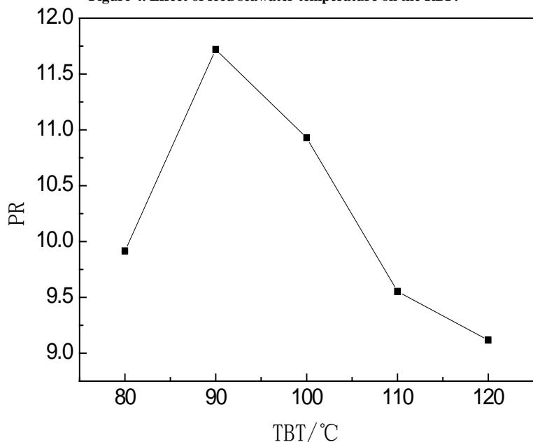
**Figure 5. Effect of top brine temperature on the PR.**
