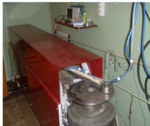
Figure 1. The appearance of the reactor. In the foreground is the engine with a crank mechanism and tension rods.
