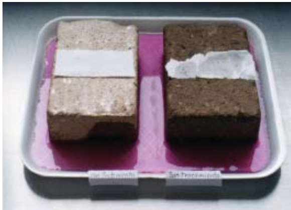
Figure 5. Bricks with and without treatment, absorbing colored solution.
