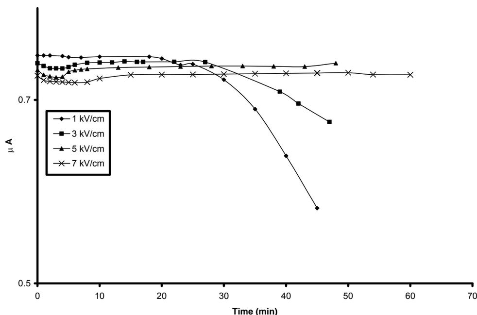
**Figure 3.** Transient current curves for BPACC sample at different applied electric fields with reverse polarity and at 300 K.
