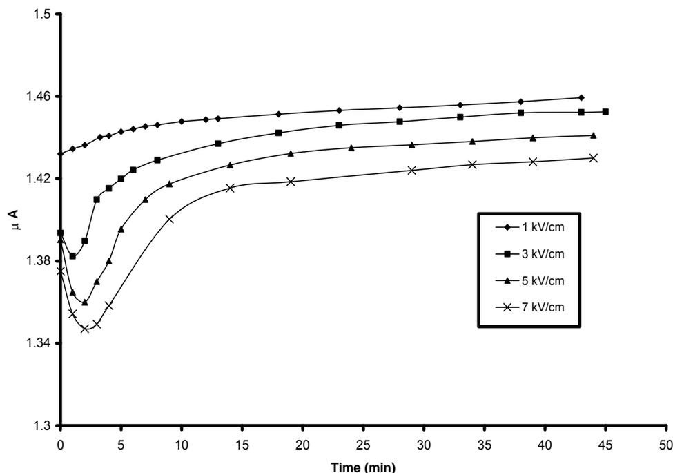
**Figure 2.** Transient current curves for BPACC sample at different applied electric fields and at 300 K.
