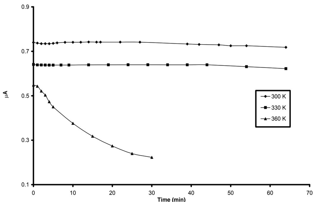
Figure 5. Transient current curves for BPACC sample at different temperatures and at electric field of 3 kV/cm with reverse polarity.
