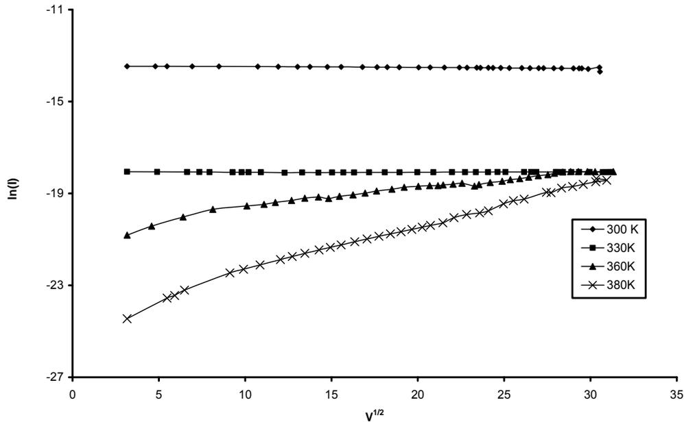
**Figure 7.  $\ln(I)$  versus  $V^{1/2}$  for BPACC at different temperatures.**
