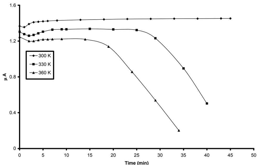
Figure 4. Transient current curves for BPACC sample at different temperatures and at electric field of 3 kV/cm.
