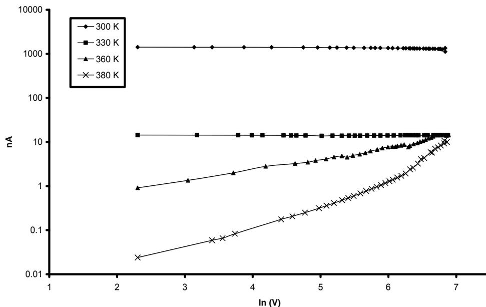
Figure 6. I-V characteristics for BPACC sample at different temperatures.
