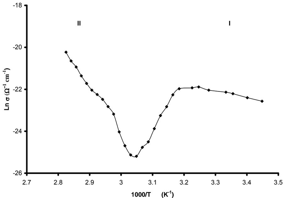
**Figure 8. Temperature dependence of dc conductivity  $\ln\sigma$  for BPACC sample.**
