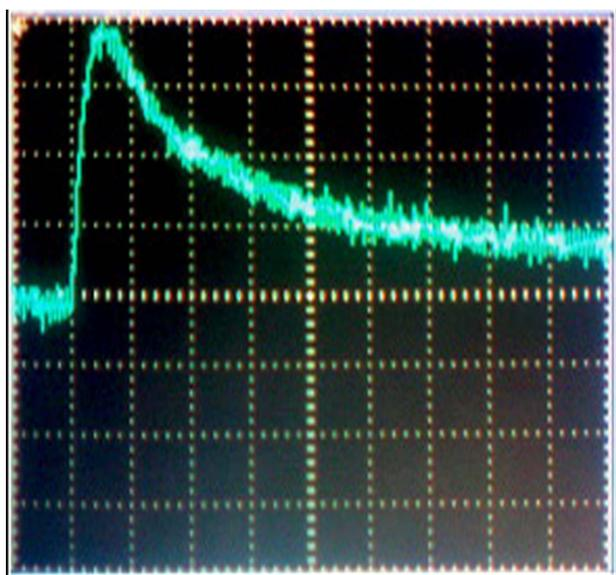
**Figure 8.** The photoresponse time of fabricated ZnO UV detector to the nitrogen laser. The time base on x-axis is 250  $\mu$ s/div.
