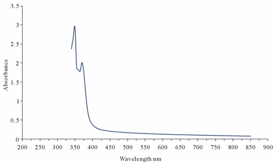
**Figure 6. The absorption spectrum of ZnO thin film on glass substrate.**
