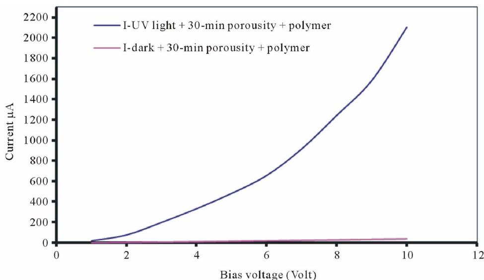
**Figure 7. The variation of the photocurrent of the fabricated ZnO UV detector on porous silicon layer as a function of the bias voltage.**
