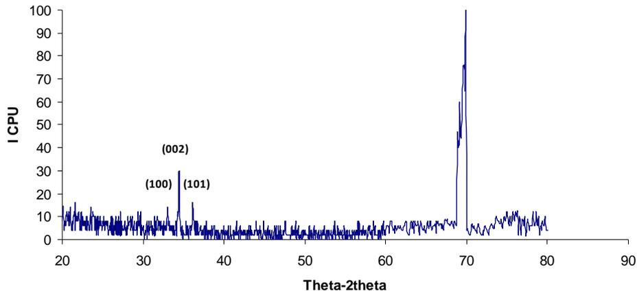
**Figure 4.** The XRD pattern of ZnO thin film on PS.
