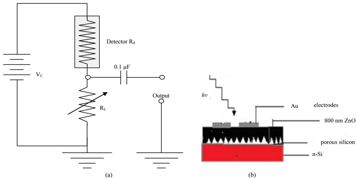
**Figure 1. (a) The operation circuit diagram of ZnO photoconductive detector where;  $R_d$  is the detector element,  $R_L$  is the load resistance and  $V_C$  is the bias voltage; (b) Schematic cross section of the fabricated ZnO porous silicon detector.**
