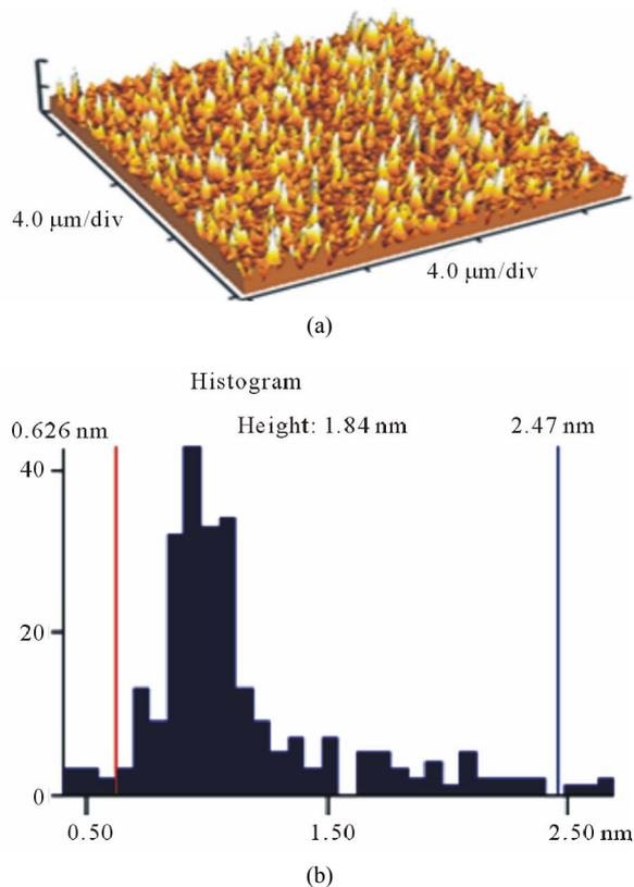
**Figure 2.** (a) Scanning probe Microscope image of porous silicon layer of 30 sec; (b) The histogram of the PS layer.
