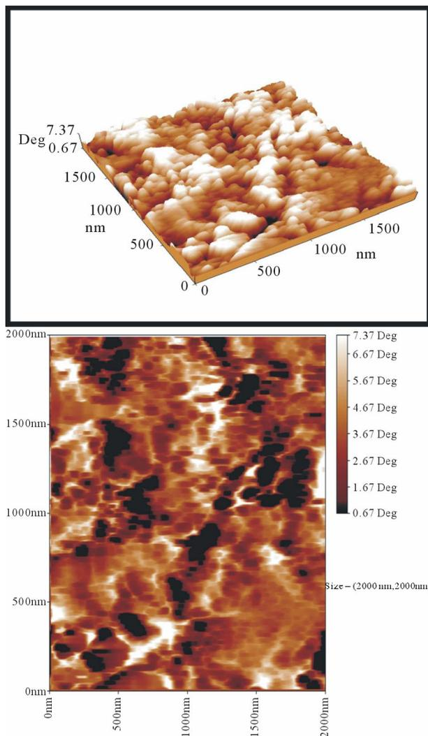
**Figure 3.** 2D and 3D Scanning Probe Microscope images of ZnO thin film deposited on PS.
