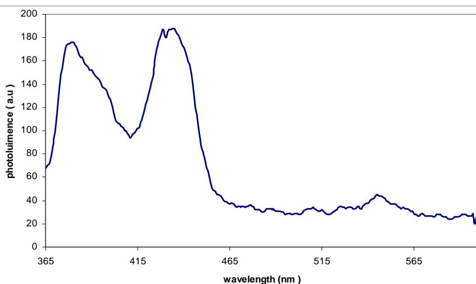
**Figure 5.** The Photoluminescence (PL) spectrum of ZnO thin film deposited on PS.
