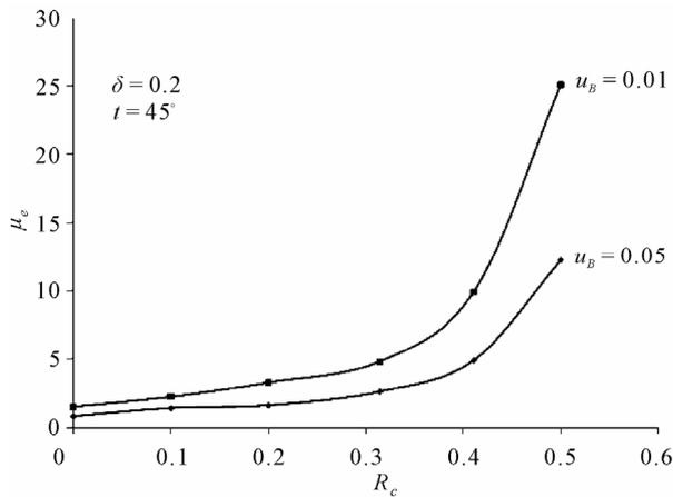
**Figure 6.** Variation of effective viscosity with catheter radius.
