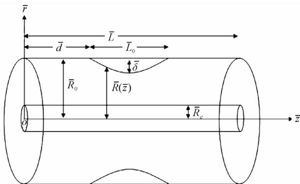
**Figure 1. Geometry of an axially symmetrical stenosis with an inserted catheter.**
