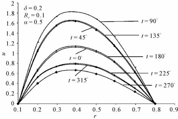
Figure 2. Variation of axial velocity with radial distance.
