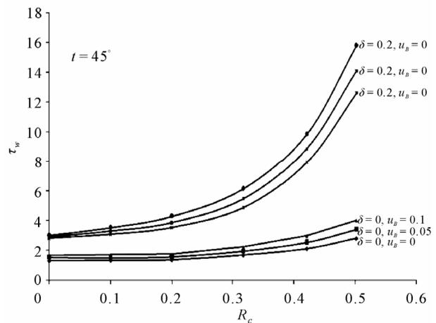
Figure 5. Variation of wall shear stress with catheter radius.
