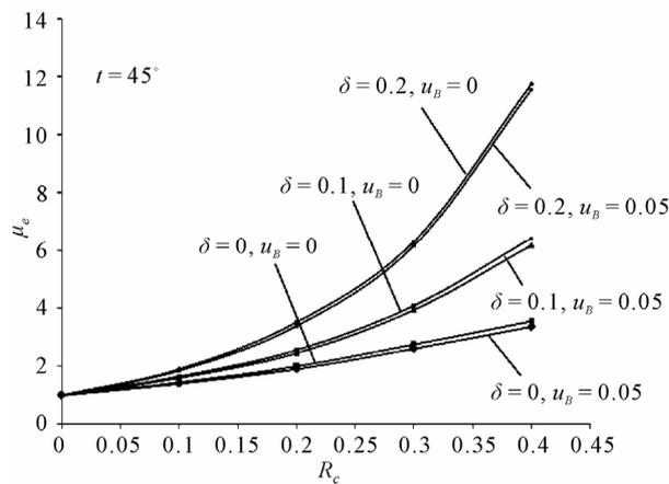
**Figure 7.** Variation of effective viscosity with catheter radius.
