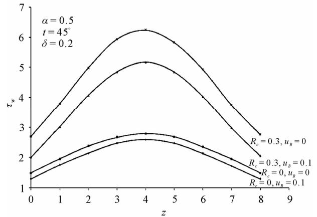
Figure 4. Variation of wall shear stress with axial distance.
