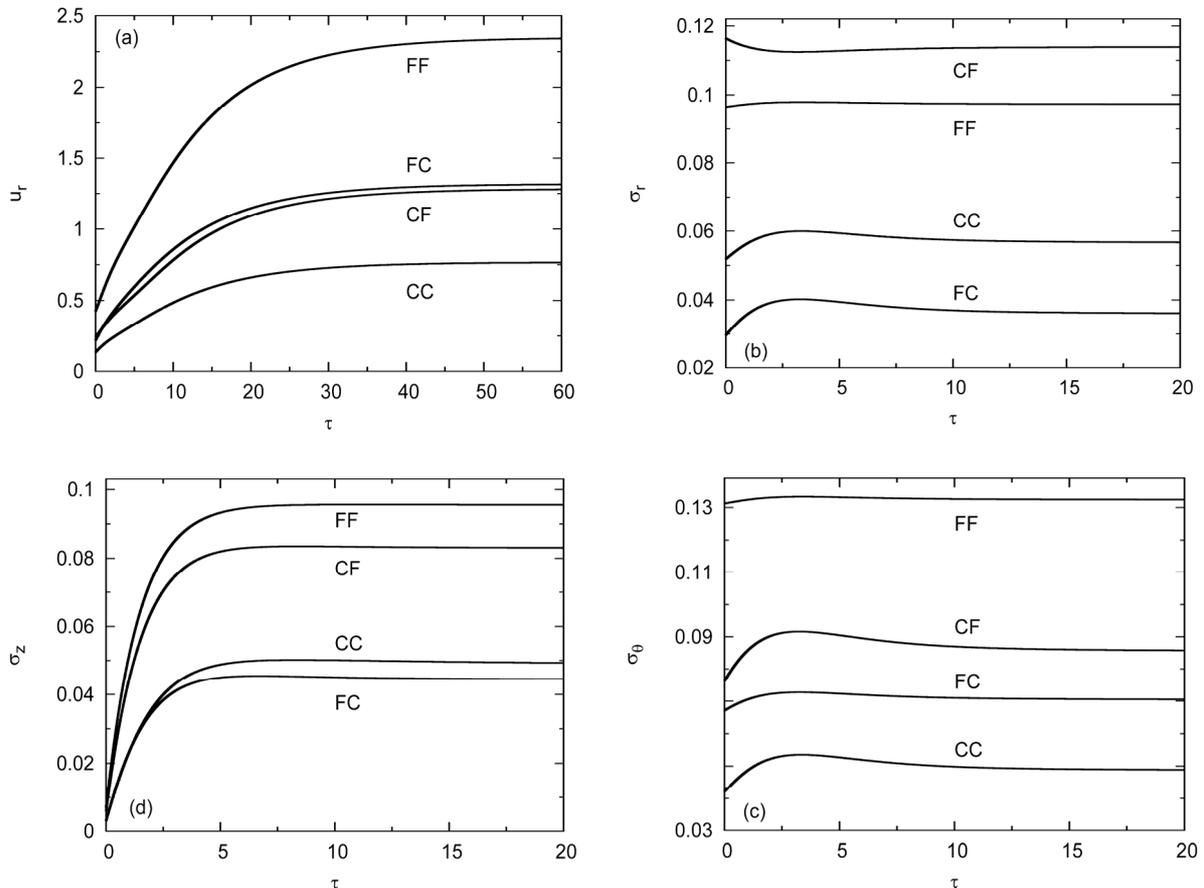
**Figure 9.** The effect of time parameter  $\tau$  on (a)  $u_r$ , (b)  $\sigma_r$ , (c)  $\sigma_\theta$  and (d)  $\sigma_z$  of a variable-thickness viscoelastic hollow cylinder at  $\bar{r} = 0.5$ .
