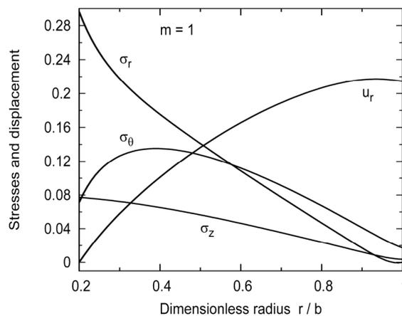
**Figure 6. Distribution of dimensionless stresses and displacement through the radial direction of a FC variable-thickness viscoelastic hollow cylinder.**
