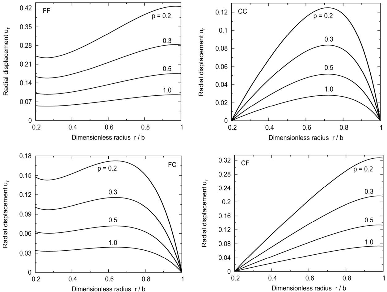
**Figure 8.** The effect of the constitutive parameter  $p$  on  $u_r$  of a variable-thickness viscoelastic hollow cylinder.
