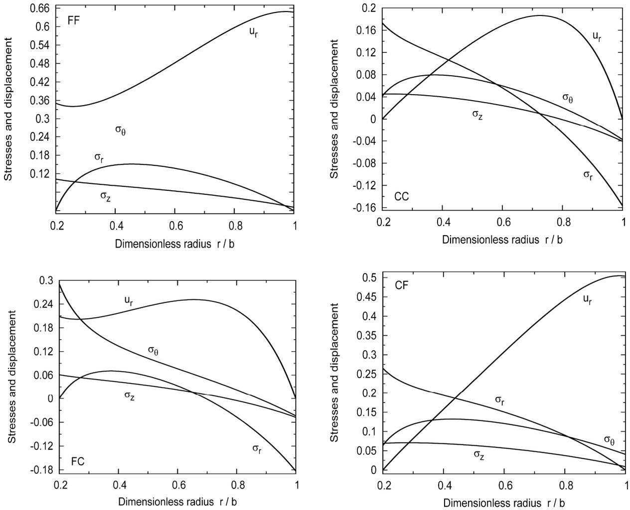
Figure 1. Dimensionless stresses and displacement for a variable-thickness viscoelastic hollow cylinder subjected to various boundary conditions ( $k = 0.6, n = 0.8, m = 0.5$ ).
