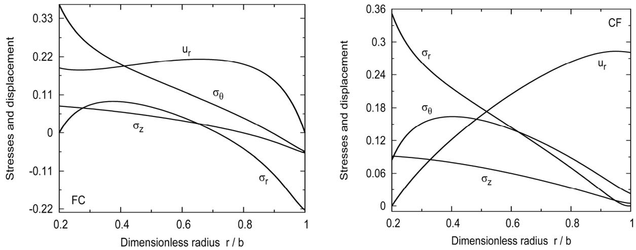
**Figure 2. Dimensionless stresses and displacement for a variable-thickness viscoelastic hollow cylinder subjected to various boundary conditions ( $k = 2.5, n = 0.8, m = 0.5$ ).**
