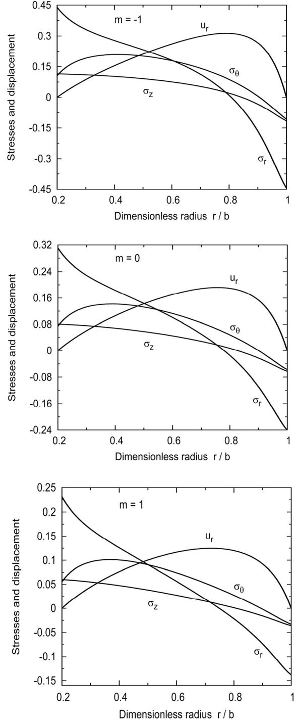
**Figure 5.** Distribution of dimensionless stresses and displacement through the radial direction of a CC variable-thickness viscoelastic hollow cylinder.
