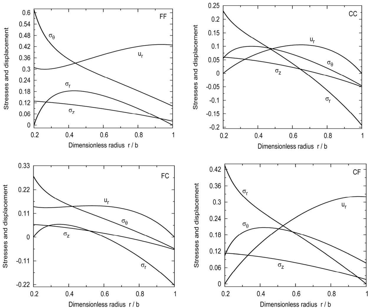
**Figure 3. Dimensionless stresses and displacement for a variable-thickness viscoelastic hollow cylinder subjected to various boundary conditions ( $k = 2.5, n = 0.4, m = 0.5$ ).**
