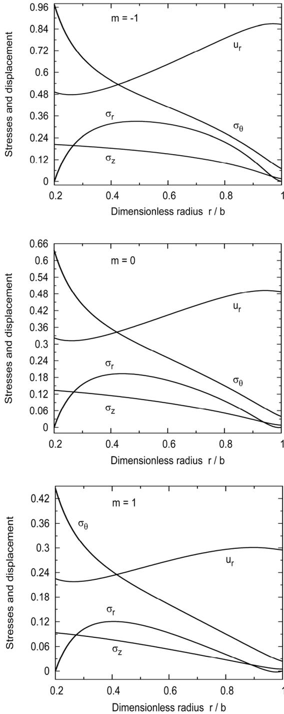
**Figure 4.** Distribution of dimensionless stresses and displacement through the radial direction of a FF variable-thickness viscoelastic hollow cylinder.
