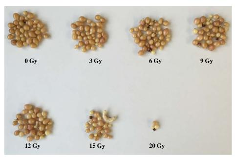
**Figure 2.** Effect of gamma irradiation treatments on micro-tuber production of *S. tuberosum* cv. Desirée (4×). The tuberization rate diminished with increasing gamma dose, with doses above 12 Gy reducing number, size and weight of micro-tubers.
