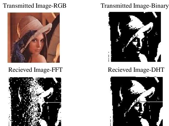
Figure 7. Transmitted & received images for FFT & DHT-OFDM using \pi/4 DQPSK over Rayleigh channel.
