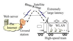
Figure 1. Configuration of target WLAN system.
