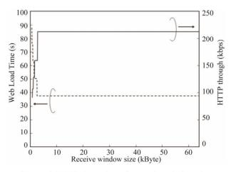
Figure 4. HTTP throughput for receive window size.
