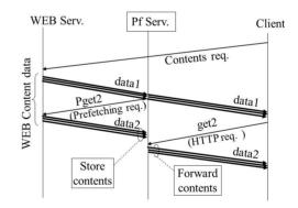
Figure 6. Signal sequence of conventional prefetching scheme.
