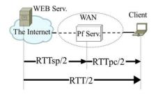
Figure 5. Configuration of conventional prefetching scheme.
