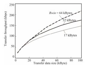
Figure 3. Transfer throughput for various data sizes and different *Rwin*.
