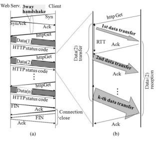
Figure 2. Sequence of HTTP (a) and data transfer procedure (b) of TCP.
