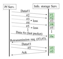
Figure 12. UDP packet loss recovery function.
