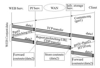
Figure 8. Signal sequence of proposed prefetching scheme.
