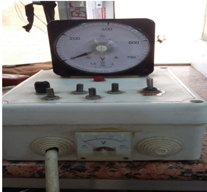
Figure 2. The electrofishing device which is used in this work is simulated to that which is used in the electricity commercial fishing.
