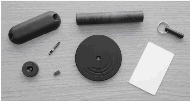
Figure 1. Examples of RFID tags for different applications.
