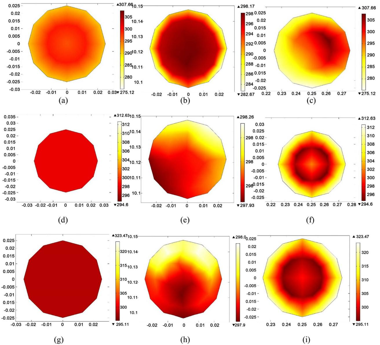
Figure 4. Temperature slice at 6.15 am: arclength (a) 5 m, (b) 10.25 m, (c) 15.5 m; at 12.00 pm: arclength (d) 5 m (e) 10.25 m (f) 15.5 m; at 3.15 pm: arclength (g) 5 m, (h) 10.25 m, (i) 15.5 m.
