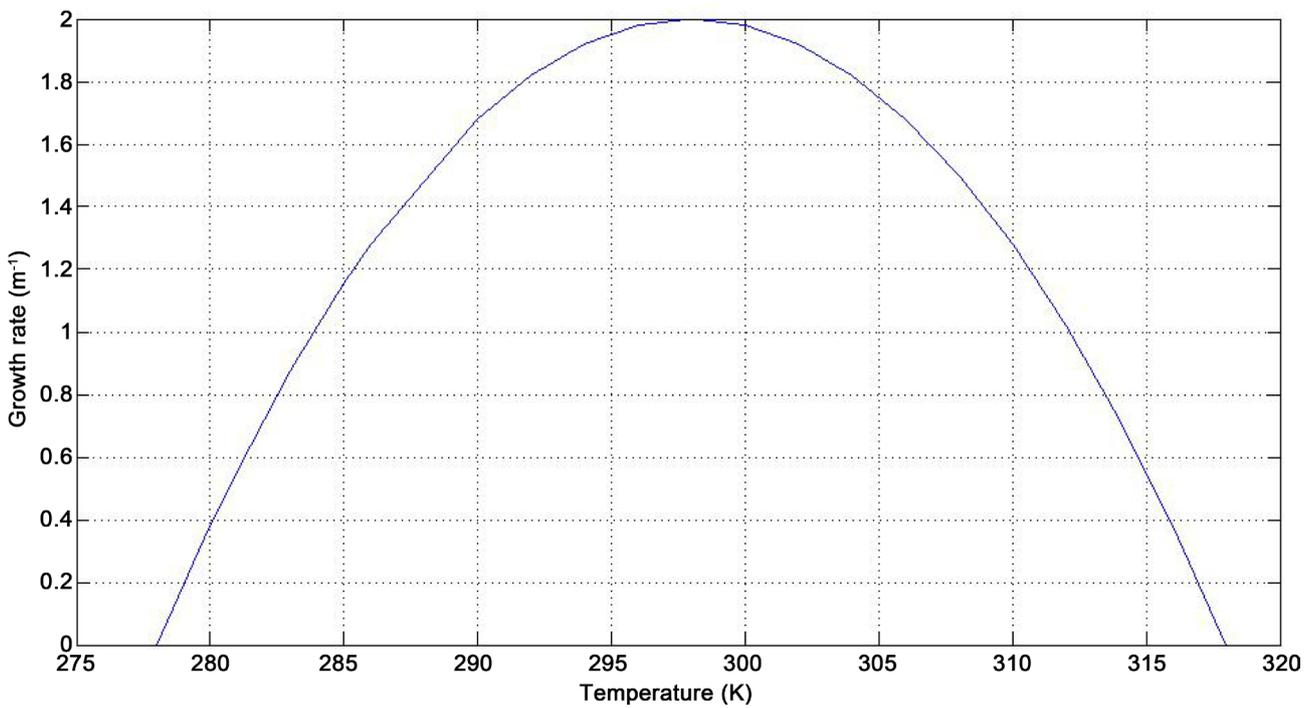
**Figure 6.** Temperature vs growth rate (m<sup>-1</sup>) (Temperatures collected from the simulation results).
