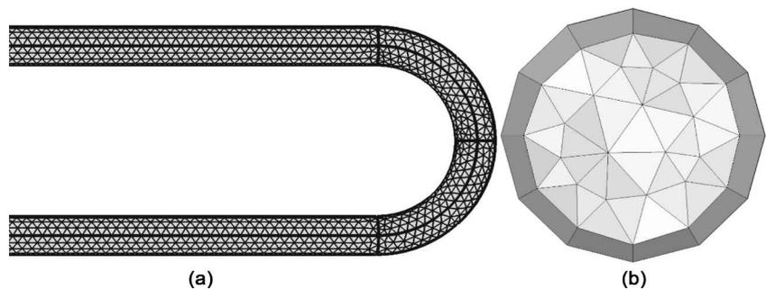
**Figure 2.** Coarse mesh design showing the (a) longitudinal view and (b) cross sectional view.
