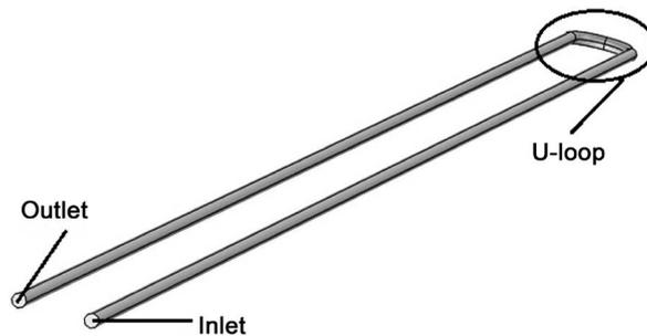
**Figure 1.** A computational domain of the HLTP showing inlet, outlet and U-loop.
