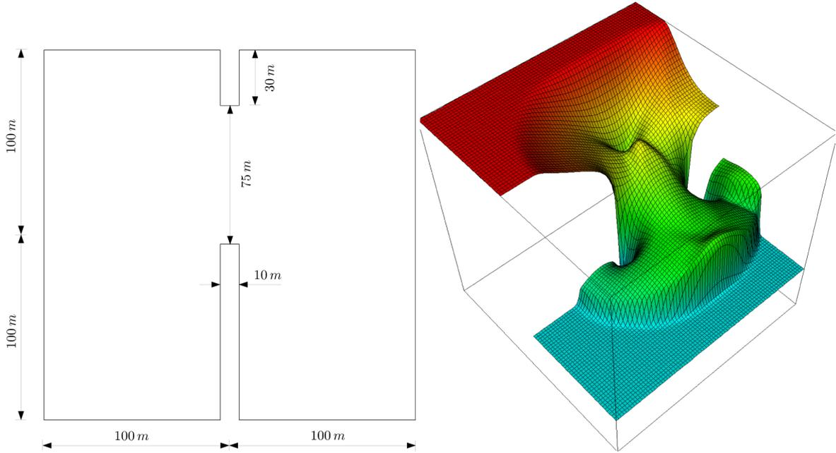
Figure 15. 2-D dam break problem. Left: geometry, right: carpet view of the water elevation at  $t = 7.2$  s.
