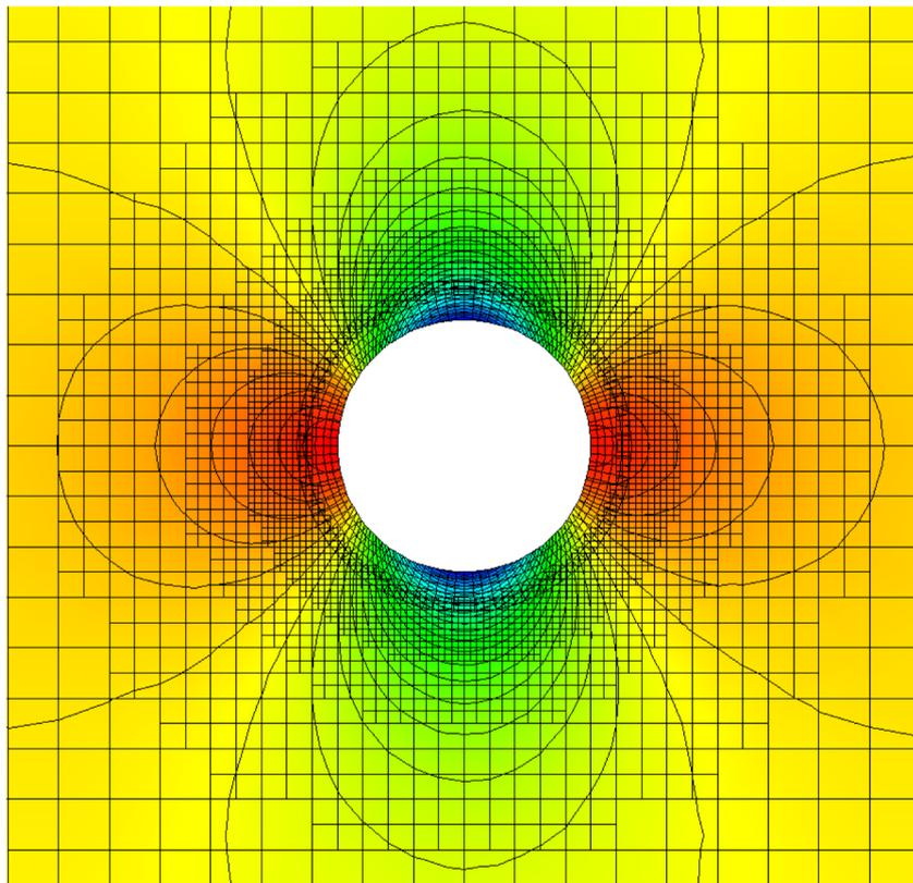
**Figure 13.** Steady pressure field of the inviscid flow ( $M = 0.1$ ) passing around a circular cylinder. The overset Cartesian and quadrilateral mesh is displayed at background.
