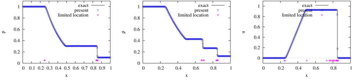
**Figure 11.**  $p_1$  solutions of Sod's shocktube problem. Left: pressure, middle: density, and right: velocity.
