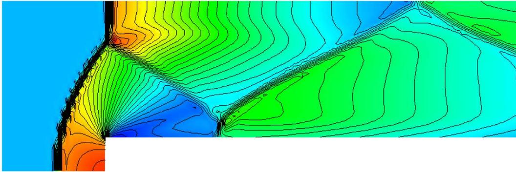
**Figure 12.** Density field of a supersonic ( $M = 3$ ) flow through a channel with a forward-facing step at  $t = 4.0$ .
