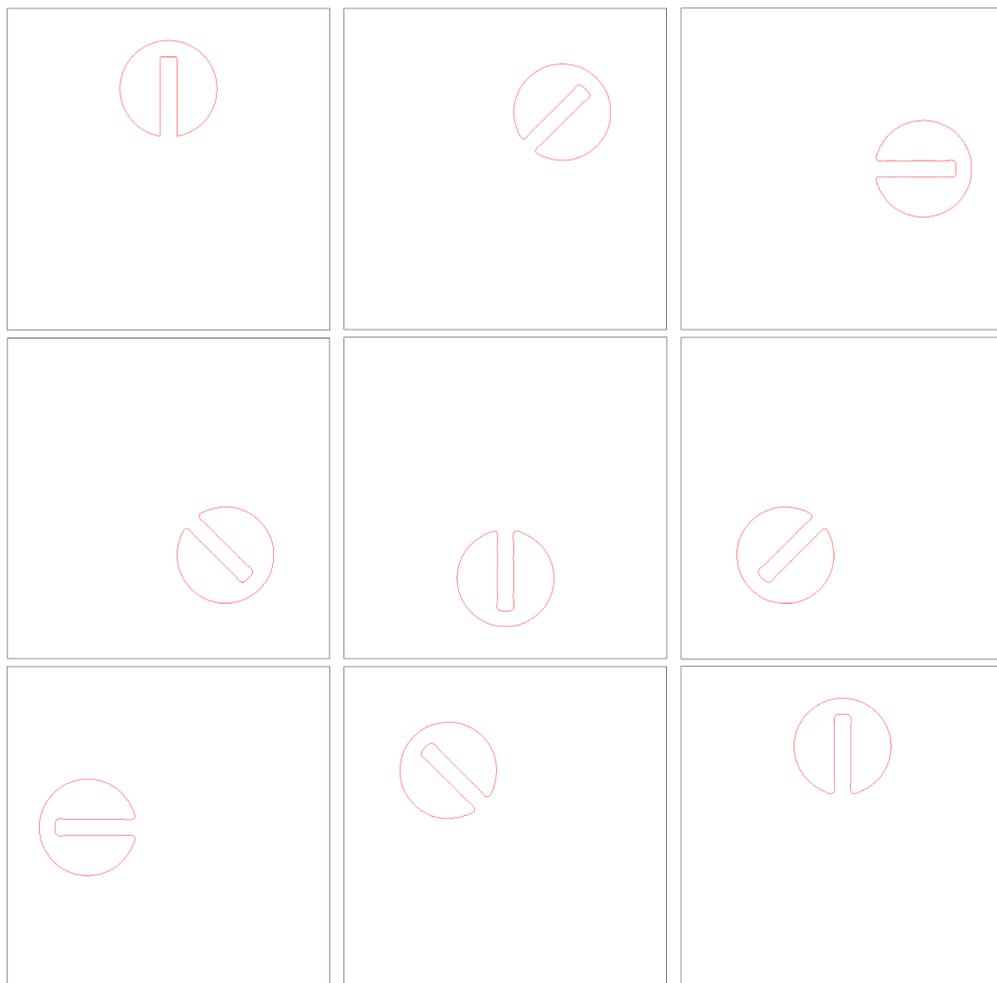
Figure 9. Rotation of Zalesak disk. The locations of the disk at several instants within one revolution. The image order is from left to right and from top to bottom.
