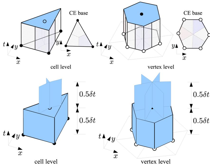
**Figure 3.** Conservation elements (CEs) and solution elements (SEs) for the triangular mesh. Top: CEs; bottom: SEs.
