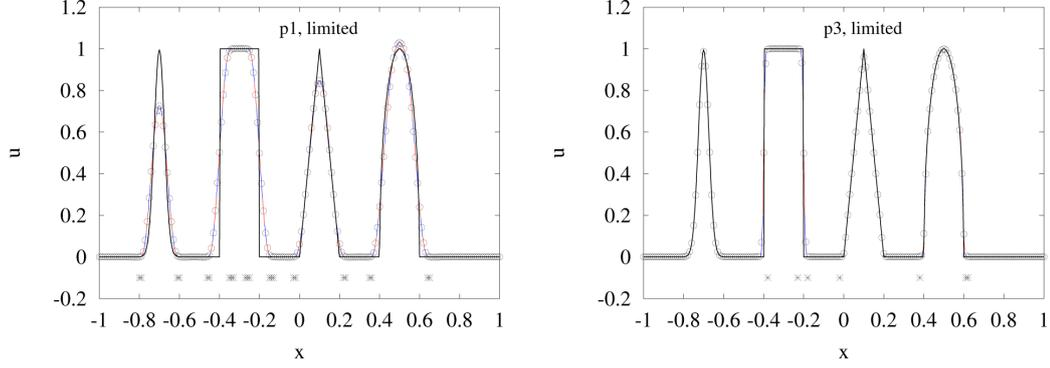
**Figure 6.** Linear advection of mixed waves. Limited solution at  $t = 8.0$ . The computational domain consists of 200 uniform elements. Thick solid line: exact solution; circles and thin colorful solid lines: current numerical solutions; and stars: oscillation indicators.
