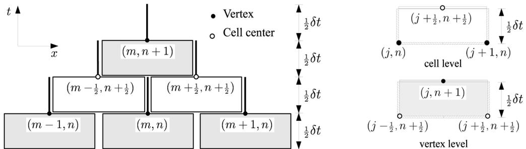
**Figure 1.** Solution elements (SEs) and conservation elements (CEs) in the  $x-t$  domain. Left: solution elements and right: conservation elements.
