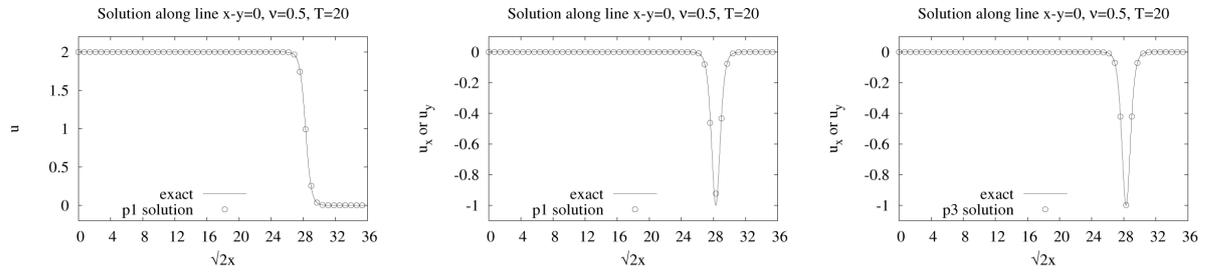
**Figure 7.** Solution of 2-D viscous Burgers equation along the diagonal line  $x - y = 0$  at  $T = 20$ . Left:  $u$ , middle:  $p1$   $u_x$  and  $u_y$ , and right:  $p3$   $u_x$  and  $u_y$ .
