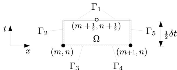
**Figure 4.** Illustration of spacetime flux conservation on a 1-D cell-level CE.
