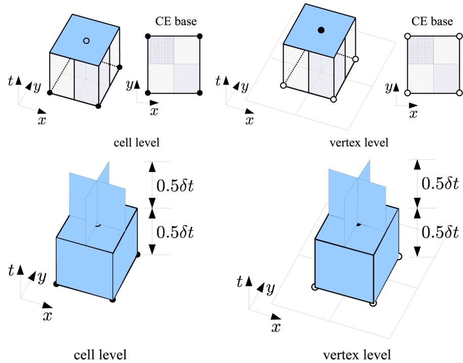
**Figure 2.** Conservation elements (CEs) and solution elements (SEs) for the quadrilateral mesh. Top: CEs; bottom: SEs.
