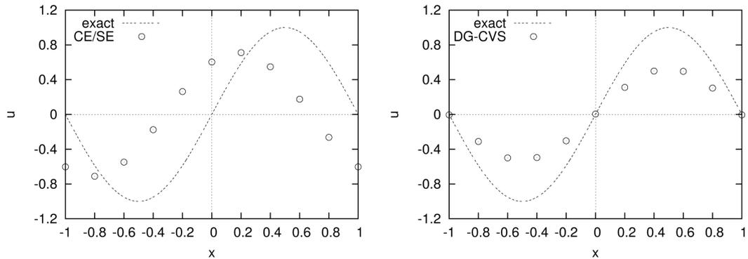
**Figure 5.** Comparison of the solutions of sinusoidal wave advection after 100 periods. Left: CE/SE. right: current method (second-order version).
