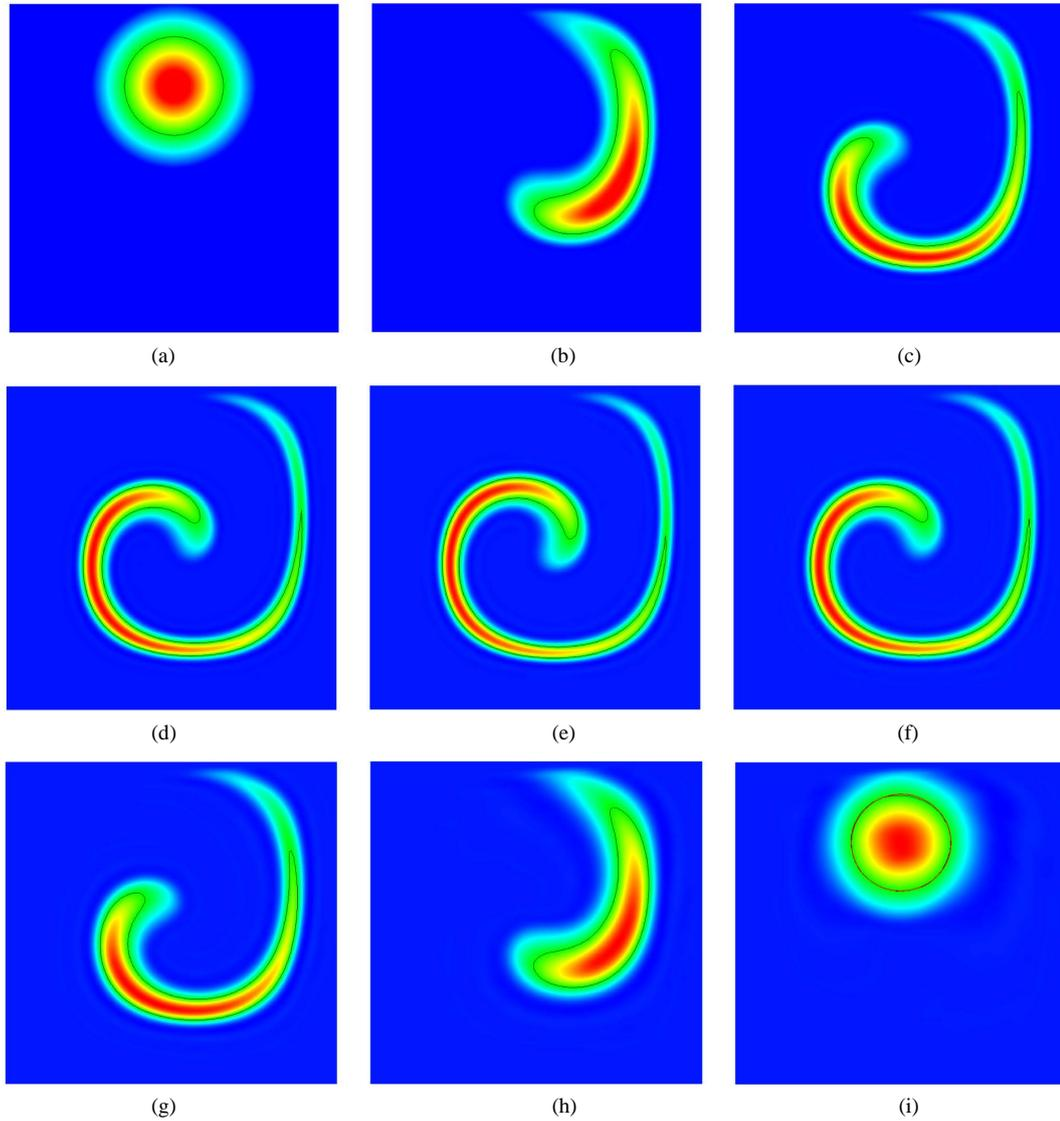
**Figure 10.**  $p3$  solution of the shearing of a circular bubble by a vortex on a  $40 \times 40$  mesh.  $T = 4$ . (a)  $t = 0.0$ ; (b)  $t = 0.5$ ; (c)  $t = 1.0$ ; (d)  $t = 1.5$ ; (e)  $t = 2.0$ ; (f)  $t = 2.5$ ; (g)  $t = 3.0$ ; (h)  $t = 3.5$ ; (i)  $t = 4.0$ .
