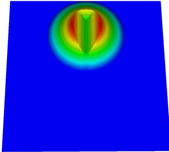
Figure 8. Zalesak disk. Initial level set is the signed distance to the disk.
