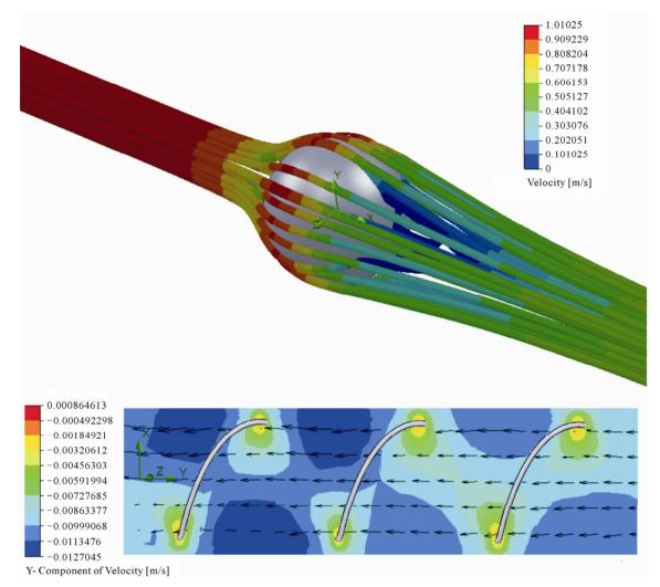
Figure 10. Top: flow trajectories past sphere at Reynolds number 150. Bottom: post processed results showing velocity contours across a cross-section of a rotating solid helix in viscous fluid at zero Reynolds number [43].
