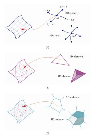
Figure 5. Discretization methods (a) FDM; (b) FEM; and (c) FVM.
