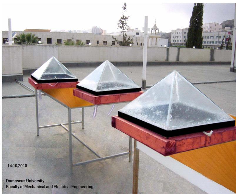
Figure 2. The fabricated solar still being tested in outdoor conditions.
