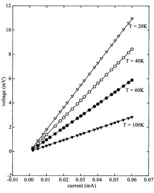
Figure 4. Voltage vs. Current data at and below 100 K.
