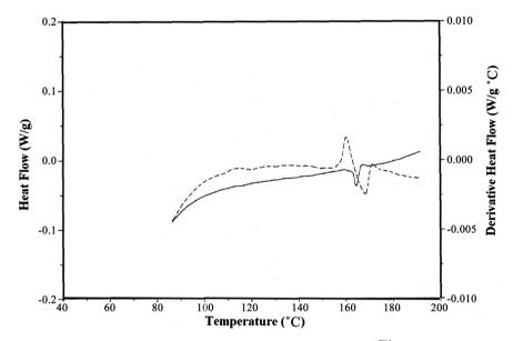
**Figure 3.** Differential Scanning Calorimetry (DSC) of Versicon<sup>TM</sup> between 90°C and 190°C, showing a crystalline transition at about 163°C. The continuous line is the heat flow and the dotted line is the derivative of the heat flow.
