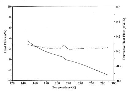
**Figure 2.** Differential Scanning Calorimetry (DSC) of Versicon<sup>TM</sup> between 150 K ( $-123^{\circ}$ C) and 290 K ( $17^{\circ}$ C), showing a glass transition at about 210 K ( $-63^{\circ}$ C). The continuous line is the heat flow and the dotted line is the derivative of the heat flow.
