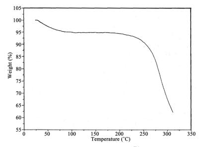
Figure 1. Thermogravimetric (TGA) Analysis of Versicon<sup>™</sup> between 25°C and 300°C.
