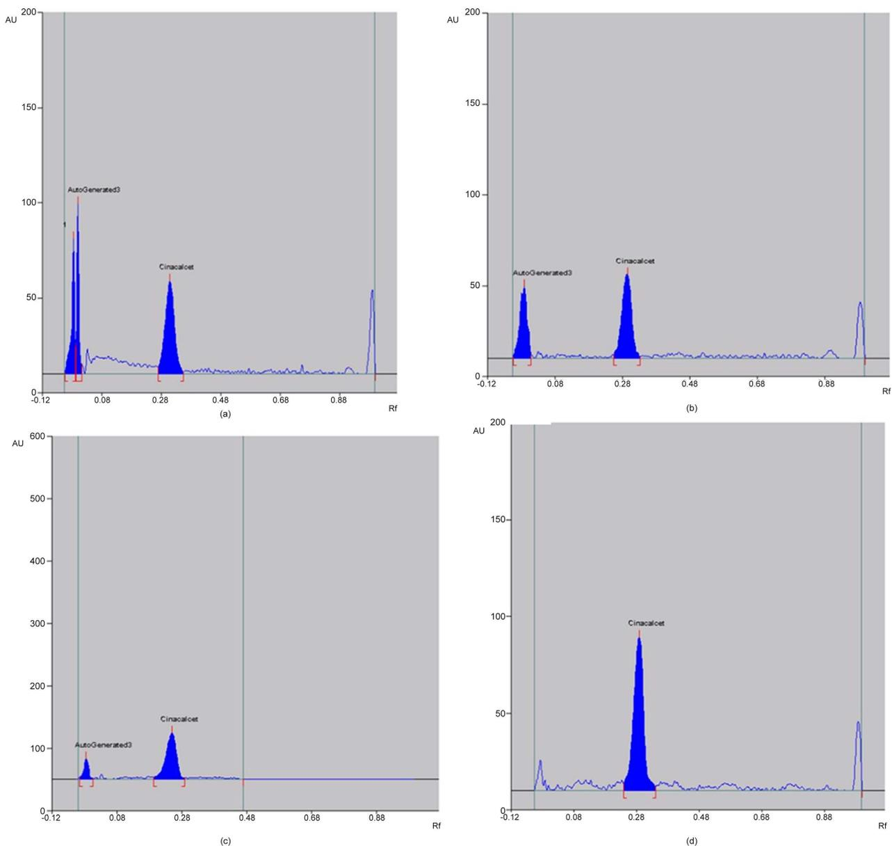
**Figure 3.** HPTLC chromatograms of cinacalcet hydrochloride obtained from degradation studies: (a) Acid degradation; (b) Alkali degradation; (c) Photo-degradation; (d) Cinacalcet API.
