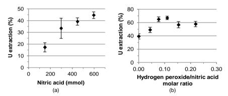
Figure 2. Influence of nitric acid quantity (a) or molar ratio of hydrogen peroxide/nitric acid (b) used for the microwave digestion of urine samples on the U extraction yield by the carboxylic calixarene column at pH 5.2. (a) Only nitric acid (10 to 50 mL of 67 wt% nitric acid) was used for the step of microwave digestion. (b) 30 mL of nitric acid (67 wt%) was used in mixture with various volumes of hydrogen peroxide (2 to 10 mL of 30 wt% hydrogen peroxide).
