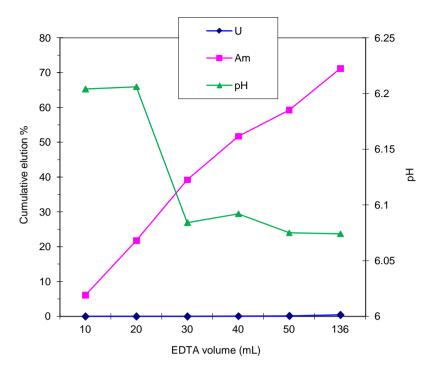
**Figure 5.** Cumulative elution yield (%) of U and Am from the carboxylic calixarene (CC) column and pH variation of EDTA solution (0.1 mM EDTA + 0.03 M sodium acetate buffer at pH 6) as a function of EDTA volume passed through the column. U and Am extraction from mineralized urines was previously performed at pH 5.2 on CC column.
