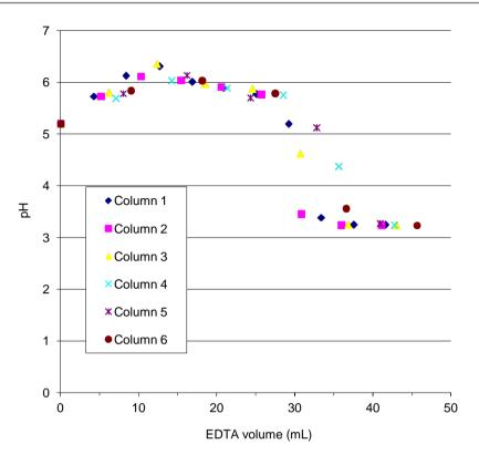
**Figure 3.** pH of EDTA eluent (0.1 mM) measured after its loading in carboxylic calixarene (CC) column as a function of its percolated volume, after U and Am extraction from mineralized urines on CC column at pH 5.2.
