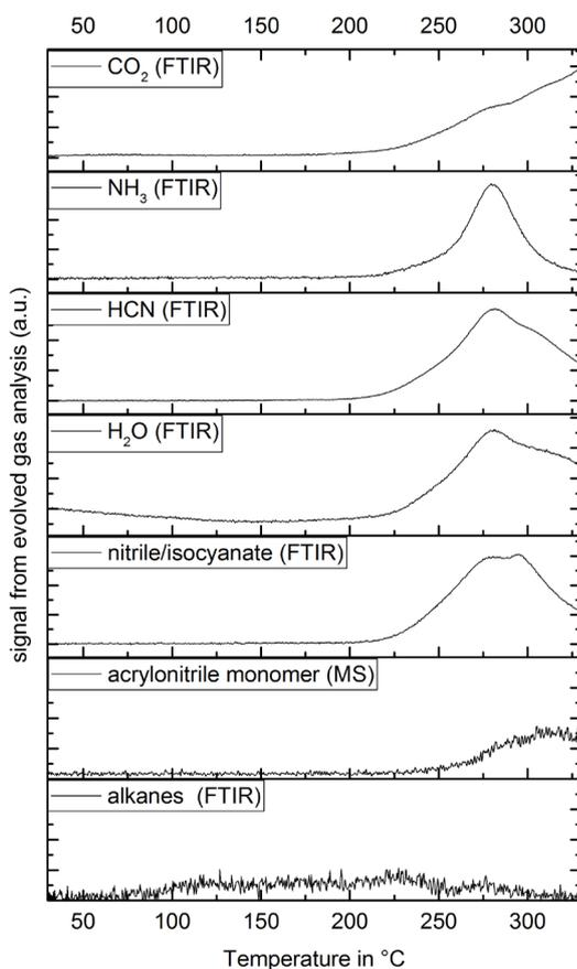
**Figure 7.** Overview of gas emissions from fiber 1 (fixed) during thermal treatment at 2 K/min.
