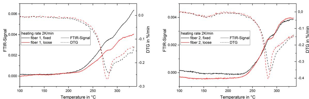
**Figure 12.** FTIR-signal of CO<sub>2</sub> in gas emission and mass change rate (DTG) during thermal treatment of fiber 1 (left) and 2 (right) at 2 K/min.
