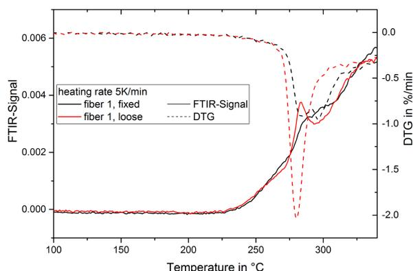
**Figure 13.** FTIR-signal of CO<sub>2</sub> in gas emission and mass change rate (DTG) during thermal treatment of fiber 1 at 5 K/min.
