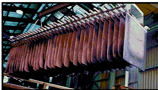
Figure 2. Scrap copper anode returned to the smelting process.
