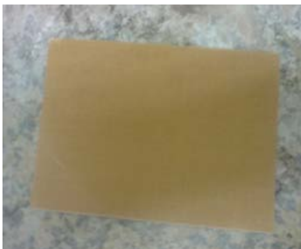
Figure 6. Cationic exchange membrane IONAC MC-3480.
