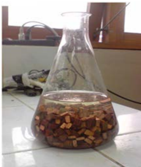
Figure 4. Scrap copper anode 1 \times 1 \text{ cm}^2 in surface and treated with \text{HNO}_3 at 10%.
