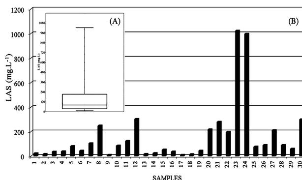
**Figure 1. (A) Box-plot of LAS from the 30 samples and (B) histogram of LAS in each sample from the commercial laundry water.**
