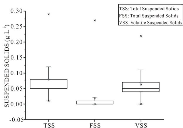
Figure 2. Solids suspended in greywater.
