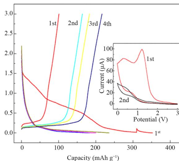
**Figure 1.** The voltage profiles of a Li/NG cell in the first four cycles using 1 M LiPF<sub>6</sub>/PC + 1 vol.% ATFEC electrolyte and cycled at a current density of 0.1 mA·cm<sup>-2</sup> between 0 and 3.0 V vs Li. The inset is for the cyclic voltammograms of a three-electrode Li/NG cell using the same electrolyte in the first two cycles at a scan rate of 0.1 mV·s<sup>-1</sup> [25].
