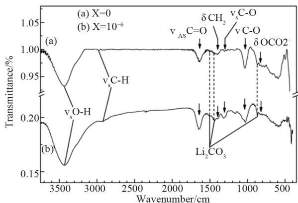
**Figure 3.** The FTIR spectra of MCMB electrodes cycled in different EC-based electrolytes: (a) without GCL; (b) with GCL [33].
