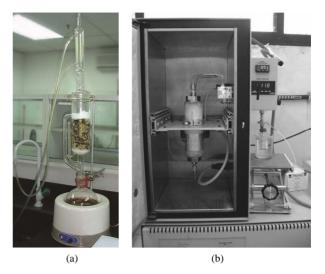
Figure 2. (a) Soxhlet for solvent extraction; (b) Supercritical extraction system SFT-150 by supercritical fluid technologies Inc. Newark, DE, USA.
