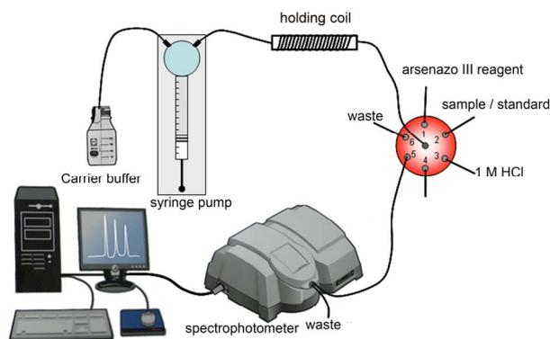
**Figure 1.** Set-up of SIA calcium assay system based on arsenazo III method.
